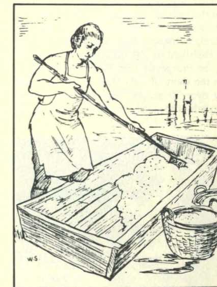
A final phase of the salt making process involved placing thick salt, obtained through boiling sea water, into wicker baskets. This allowed excess brine to drain away. This illustration, by Toms River artist Wini Smart, appeared in Pennsylvania Salt Works at Shelter Cove published by Pauline S. Miller, also of Toms Creek.
